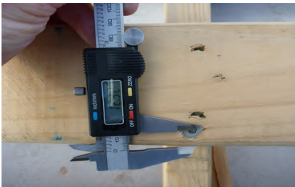
Figure 15. Photograph showing a batten non-compliant screw close to the edge of the batten
